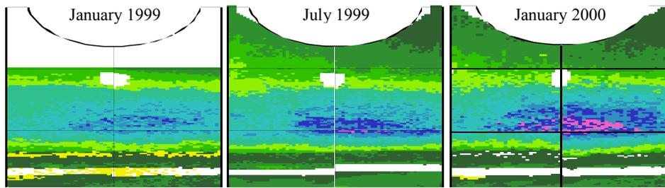
The MicroMap system enables difficult access or awkward geometry components to be inspected by ultrasonic C-scan or corrosion mapping. This includes elbows, Tees, manifolds, sumps, dished ends, nozzles, etc. The system also maintains a record of the area covered, thereby providing assurance of a greater coverage than generally achieved by conventional manual ultrasonic inspection.
